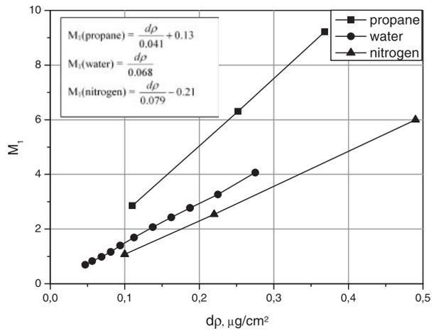
Figure 5. First moments  $M_1$ , of the calculated cluster size distribution for liquid water and the experimental cluster size distributions for nitrogen and propane.
