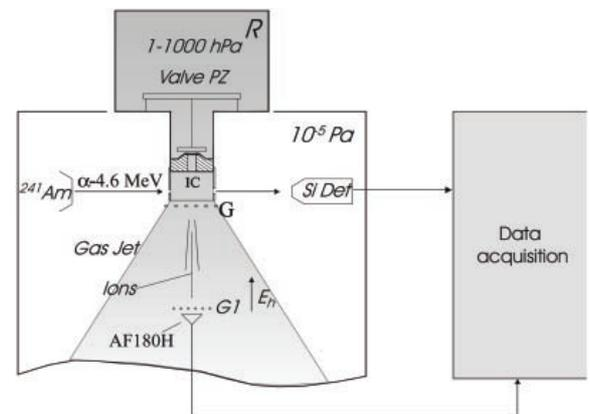
Figure 3. Schematic view of the Jet Counter: configuration for the experiments with alpha particles, PZ- piezoelectric valve; AF180H- ion detector, Si alpha particle detector, IC interaction chamber.
