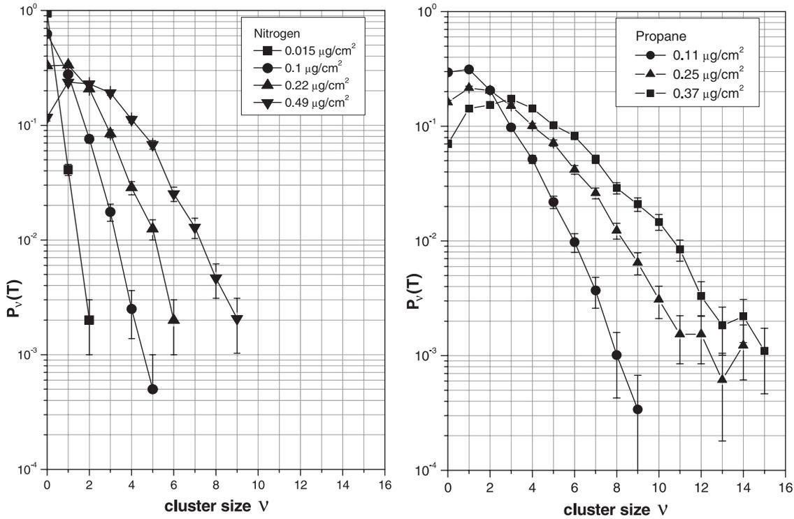
Figure 4. Experimental frequency distributions of ionization clusters for different target diameters for nitrogen and propane, irradiated by 4.6 MeV alpha particles. For propane the energy of alpha particles is attenuated by Mylar foil ( $1 \mu\text{g cm}^{-2}$ ).
